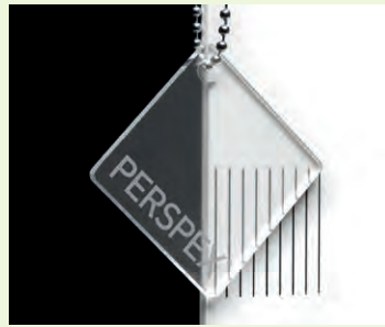
Colour: Clear Code: SA 000 Dimensions(mm): 3050 x 2030 Thickness (mm): 3, 5, 10 Light Transmission (%): 91
