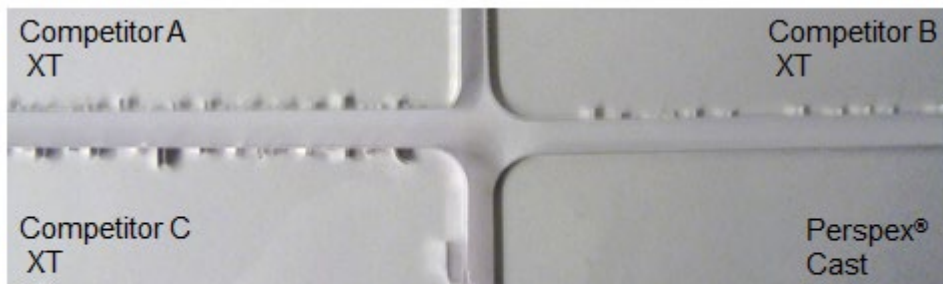
Chemical Resistance Comparison (samples laser cut and exposed to isopropyl alcohol for 30 minutes)
